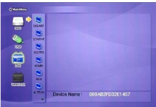
① [Mode Selection] Select 'LAN' icon and press [OK]. (In case of wireless network, select 'WIRELESS' icon,
